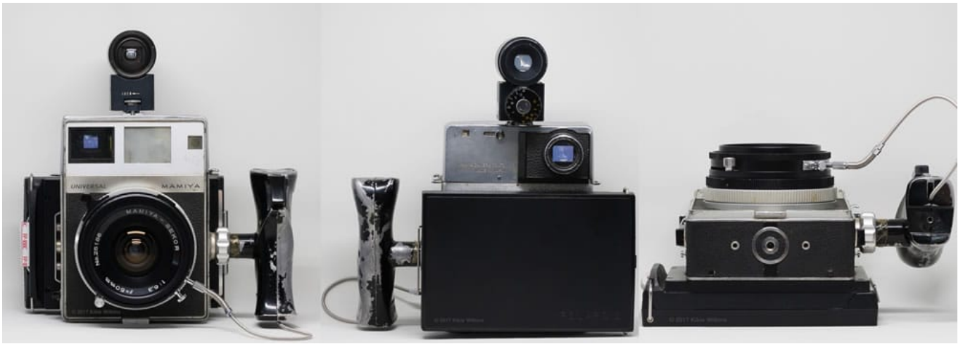
Mamiya Universal Press with Type-2 Polaroid instant film back and 50mm f/6.3 lens with accessory viewfinder
